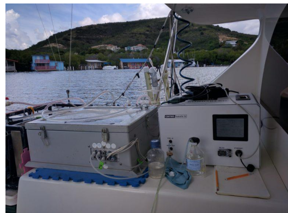
Fig. 5 Flow-through system to measure several chemical parameters (photo credit: Chris Hunt)
