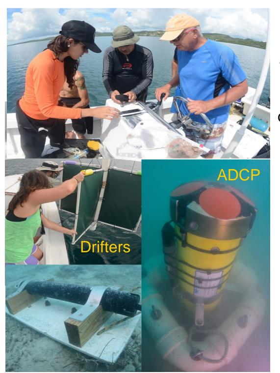
Getting ready to deploy a set of ADCPs and drifters to characterize the surface currents in the study area.
