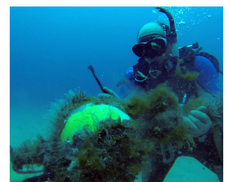
Probing the internal structure of plunging waves using inertial drifters (Amador & Canals, 2015)
