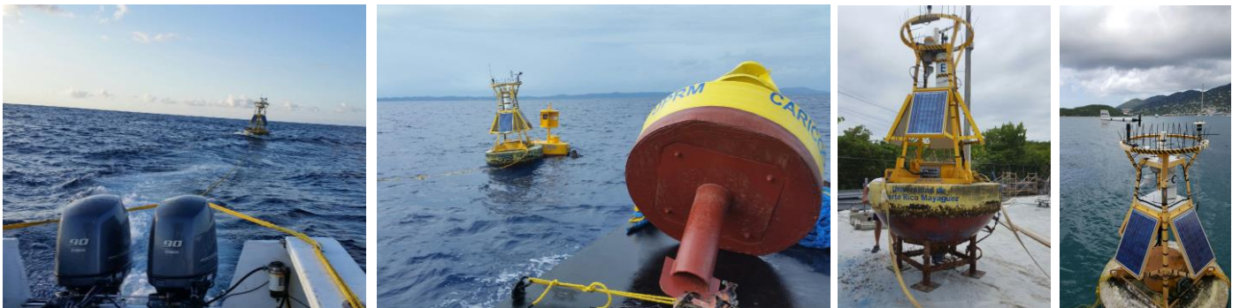
Fig. 2 Photographs of CARICOOS buoys during the yearly maintenance.
