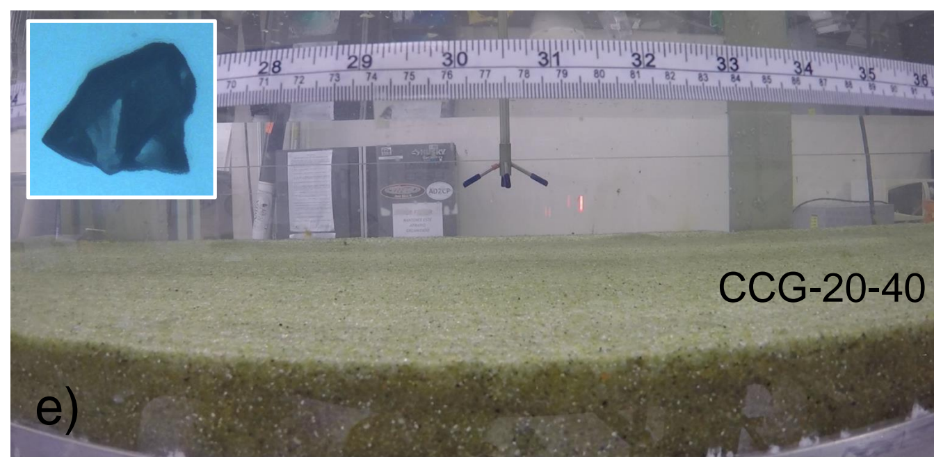
a) Example of ripples developed during the trials. b) GoPro setup. c) Ripples formed by an oscillating motion of with T=20s and amplitude A=65cm. The separation between crest ( \lambda ) is 4cm. d) Same as c) with T=15s, A=75cm, and \lambda=8 cm. e) For self-similar conditions ripples did not develop for CCG-20-40 particles, due to their high angularity.
