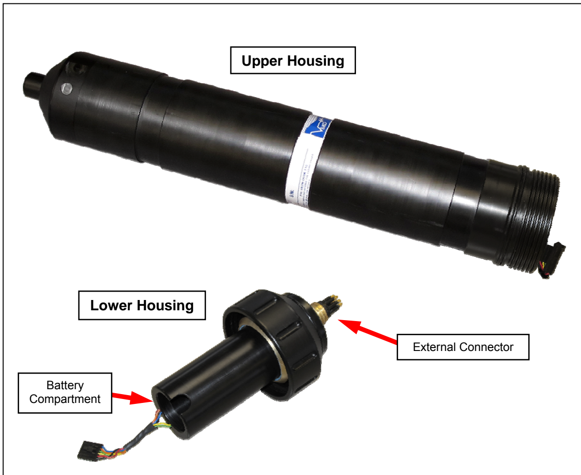
A VR2C-69kHz with lower housing removed.
