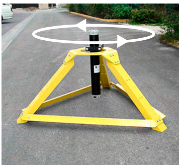
Rotate the entire system slowly around the z-axis of the Aquadopp Profiler. Turn to Chapter 4 for a definition of the z-axis.
