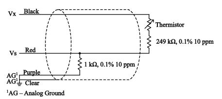
FIGURE 8-1. 107 thermistor probe schematic
