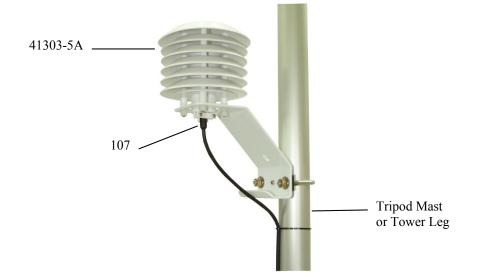
FIGURE 7-1. 107 and 41303-5A Radiation Shield on a tripod mast
