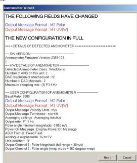
Wind will report Setting Up Anemometer and then re-start the anemometer scrolling data in UV mode.
